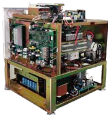
32kW / 40kW Super Capacitor Bank (PSU Generator)
